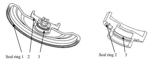
Figure 9-1 Seal rings of rotor
