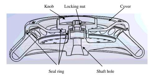
Figure 11-1 The rotor structure
