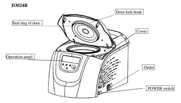
Figure 5.3 D3024R Front view of centrifuge
