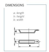
Nahita offers this small combustion boat made of unglazed porcelain which allows it to support extreme temperatures up to 1350°C. Ideal for calcination processes and for metal casting.
