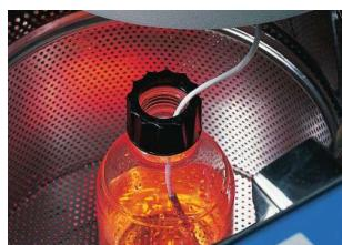
**Pt 100 Sensor.** 2<sup>nd</sup> Probe for reading sample temperature.
