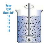
Dynamic radial flow, diagram showing the principal of agitation through a cone within the liquid. Representative of the Visco-Jet®. Rotors. Excellent results for minimum power consumption.
