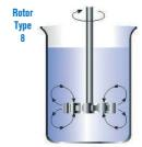
Radial flow, diagram showing the agitation within the liquid. Representative of radial turbine rotors that run parallel to the stirring axis.
