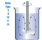
Axial flow, diagram showing the agitation flow. Representative of rotors with blades angles of 90° in relation to the stirring axis. (Rotor type; Helix).
