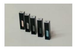
1 | Solid filter to verification of the wave-length precision in the visible rank and UV (from 329 nm to 875 nm) and for verification of the photometric accuracy.
